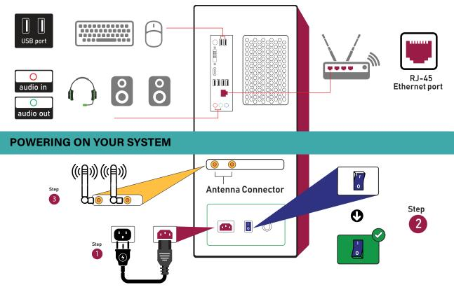
Use the included power cord and connect the cable to your system's power supply and the other end to a wall outlet
